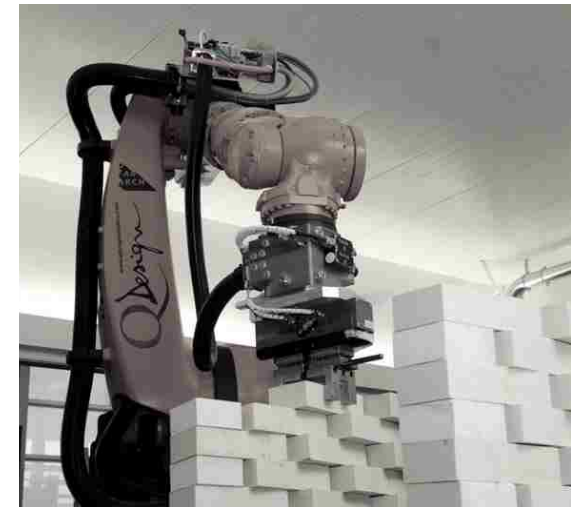
fig. 3.4 Robot brick assembly construction, by G&K
